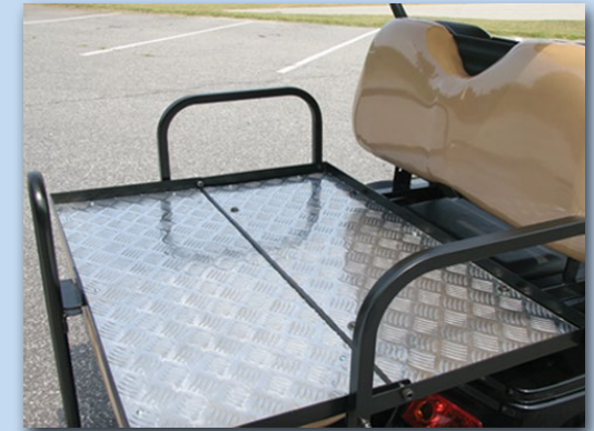
Flip seat with aluminum plate
