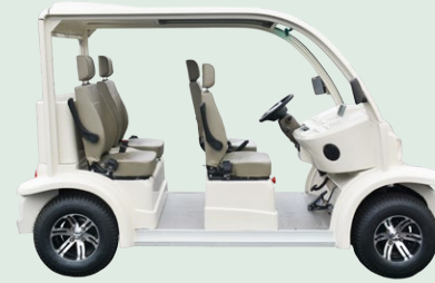
Open seating area with adjustable arm rests and seat backs (AP48-04 shown)
