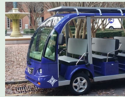
Roof-mounted solar panels (custom color shown)
