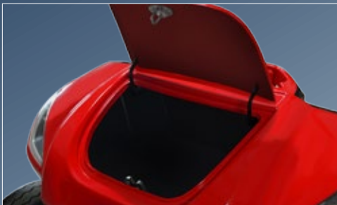
Front trunk storage space with locking electronic latch
