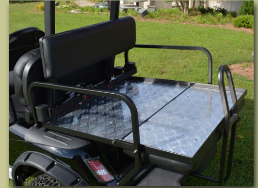
Rear flip seat: diamond-plated aluminum, 350 lb load capacity
